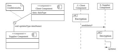
Fig. 5. Enabling Data Confidentiality mechanism
