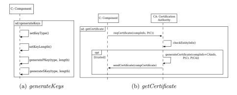
Fig. 2. UML Sequence Diagram of some preliminary operations
