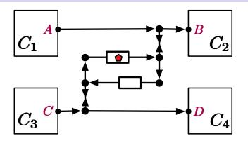
alternating data flow between  $C_1$  and  $C_2$  via AB and between  $C_3$  and  $C_4$  via CD
