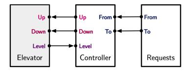
$$\begin{split} &\text{port set } \mathcal{N} = \{\text{Up}, \text{Down}, \text{Level}\} \\ &\mathcal{N}_{\mathrm{in}} = \{\text{Up}, \text{Down}\}, \, \mathcal{N}_{\mathrm{out}} = \{\text{Level}\} \\ &\mathcal{D}\textit{ata} = \{1, 2, 3\} \quad \text{three floors} \end{split}$$
