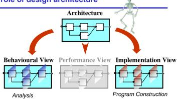
We consider that the models for analysis and the implementation should be considered as elaborated views of this basic design structure.
