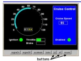
When the car ignition is switched on and the on button is pressed, the current speed is recorded and the system is enabled: it maintains the speed of the car at the recorded setting.
