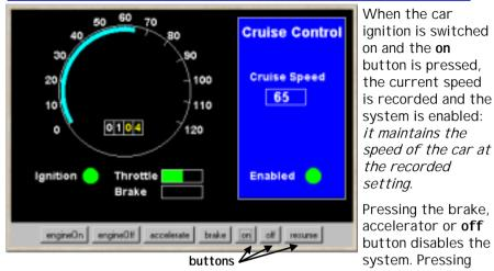
speed of the car at the recorded settina. Pressing the brake, accelerator or off button disables the system. Pressing resume or on re-
