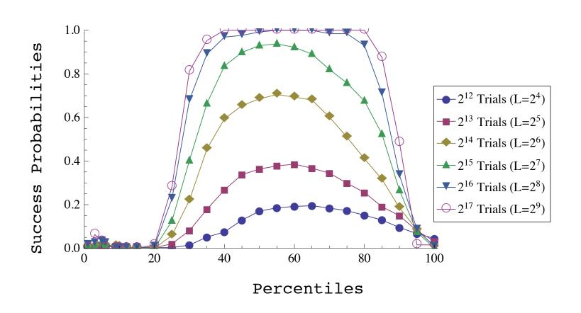
OpenSSL: recovering last byte in a block, using percentile test to extract correct byte value, no assumptions on plaintext.
