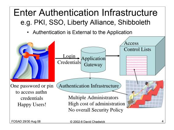
By removing the authentication function from all applications and giving it to an outside entity, we can provide the users with single sign on. PKIs with application gateways that check the user's signatures, can be one way of providing single sign on. The users are much happier when they have single sign on, since they only need to know a single password to access their credentials.
