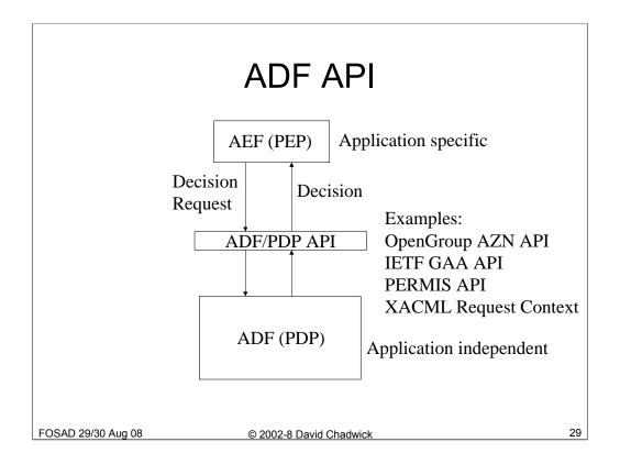
When policy based access controls are implemented, the ADF needs to have access to the policy. It would be useful if one policy and one ADF could be used by multiple targets. It would also be useful if you could build an application without having to re-implement the ADF each time.
