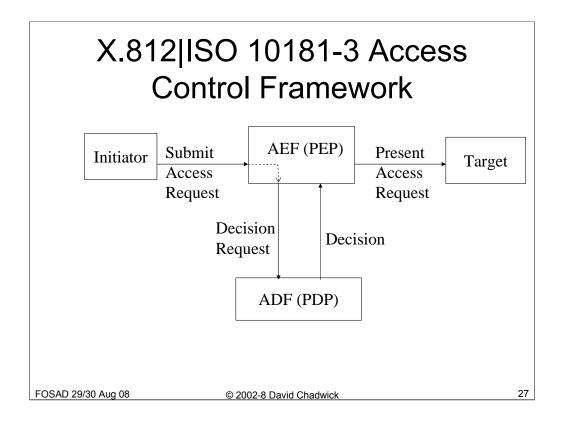
ISO 10181 specifies a standard framework for controlling access to target resources. The access control function is split into two components, the Access Control Enforcement Function (AEF) and the Access Control Decision Function (ADF). The former is responsible for enforcing the access controls, whilst the latter is responsible for making the decision about whether access can be granted or not.
