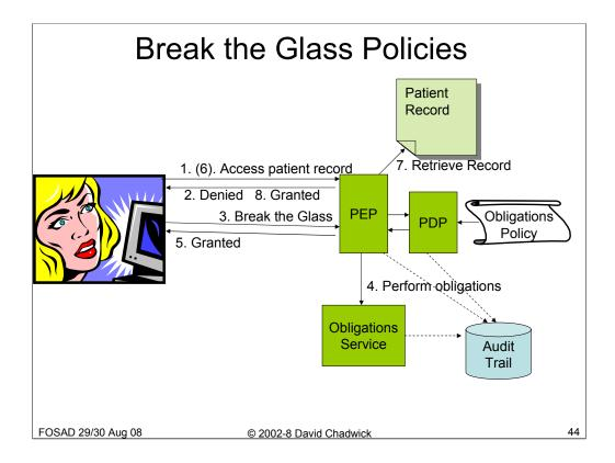
Break the Glass is both a resource (Boolean can be set to True from initial value of False) and a condition on access. In order to access the resource "Break the Glass" any conditions can be set in the Access Control Policy, including any LoA value and user roles/attributes. The granularity of the resource can be one BTG per user, one per resource, one per domain etc. We have fully described this in our paper at the Policy 2006 conference.
