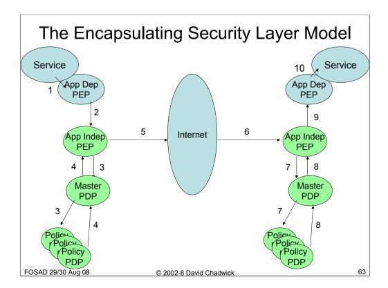
An example of this approach is SSL/TLS, which carries application layer data and protects it whilst in transfer. However, in this case the security layer will also carry authorisation policies and obligations between systems to ensure end to end enforcement of security policies. It can also perform the trust negotiation prior to establishing the service connection.
