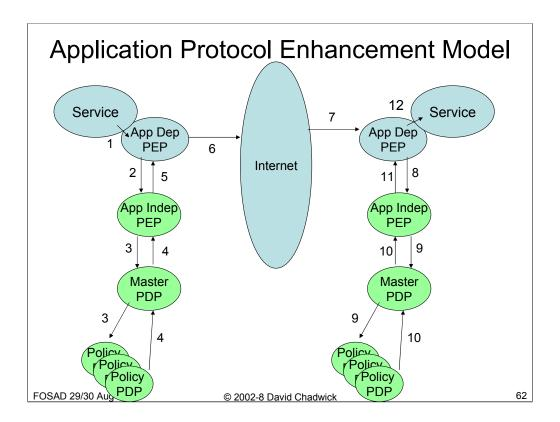
An example of this strategy is S/MIME which has enhanced the MIME protocol to carry secure email messages. It is quite simple to integrate sticky policies into S/MIME messages as attributes that can be carried along with the messages. However it cannot perform trust negotiation
