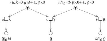
Note that E has been initially decomposed into two sequential subterms due to the presence of an occurrence of the parallel composition operator; a place has been associated with each of these sequential subterms.
